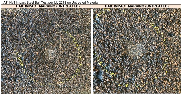
A8 Hail Impact Steel Ball Test per UL 2218 on Untreated Material
